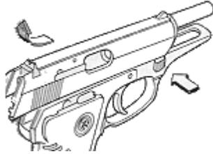
**1.** To field-strip the CZ Model 50, first remove the magazine (42) and clear the chamber. While pressing the takedown catch (35) to the left, pull the slide (1) back and lift it upward at the rear. Then ease the slide forward off the barrel (43) and remove the recoil spring (10). **2.**
