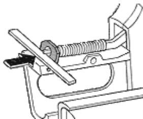
**4.** Before attempting disassembly of the lock mechanism, remove the grip screw (15) and grips (14) (27). Then carefully clamp the receiver (41) in a vise with padded jaws. Place a thin metal bar against the bottom of the spring retainer (26), and push on the bar until the retainer is free of the receiver. then ease the bar back to original position and remove the hammer spring (25) from the
