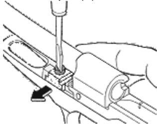
Push the takedown catch all the way to the left, and unscrew the takedown catch screw (34). In doing this, a screwdriver with a thin shank is required to clear the barrel. After removing the screw, shake out the catch and spring to the right. The hold-open latch and ejector (12) and latch spring (11) can be removed by driving out the hold-open hinge pin (13) to the left. Do not remove these unless necessary.
