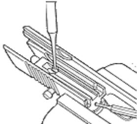
Hold the slide bottom side up in a vise. Depress the firing pin lock (9) with a punch and use a long thin punch from the front to push the firing pin lock and spring are removed, drive out the extractor pin (2), and remove extractor (6), extractor spring (5), and cartridge indicator (3). **3.**
