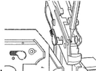
the trigger bar (28), trigger (30), hammer (23), and other lock parts.
